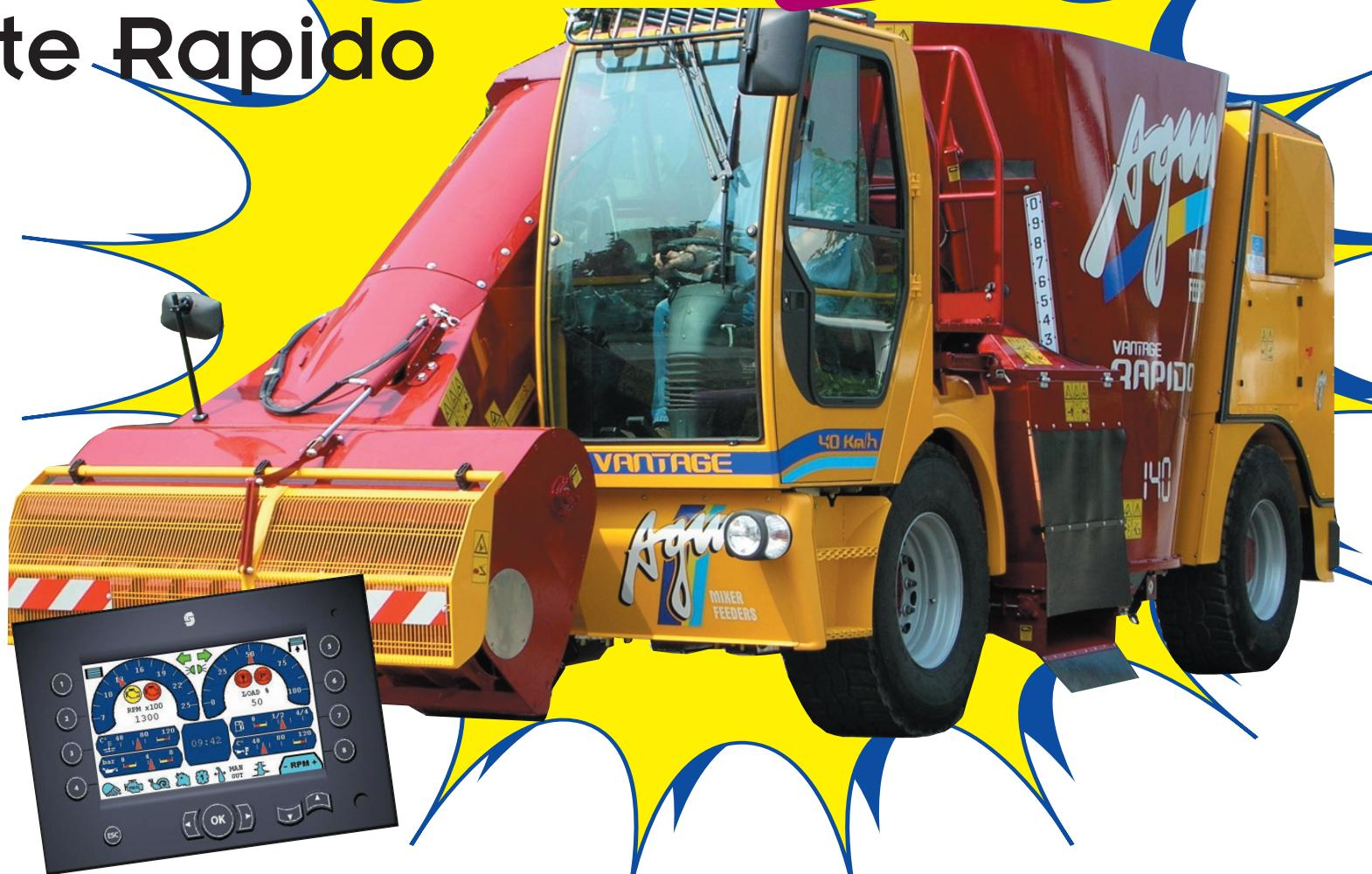
most extreme conditions and for high speed long distance driving. Its driving system, with a self-blocking 2 speed differential, along with 4 big size wheels (116 cm), allow the machine to get good performances even on iced and slippery grounds. The front axle is equipped with disc brakes with 4 hydraulic calipers to ensure a prompt and safe braking.
